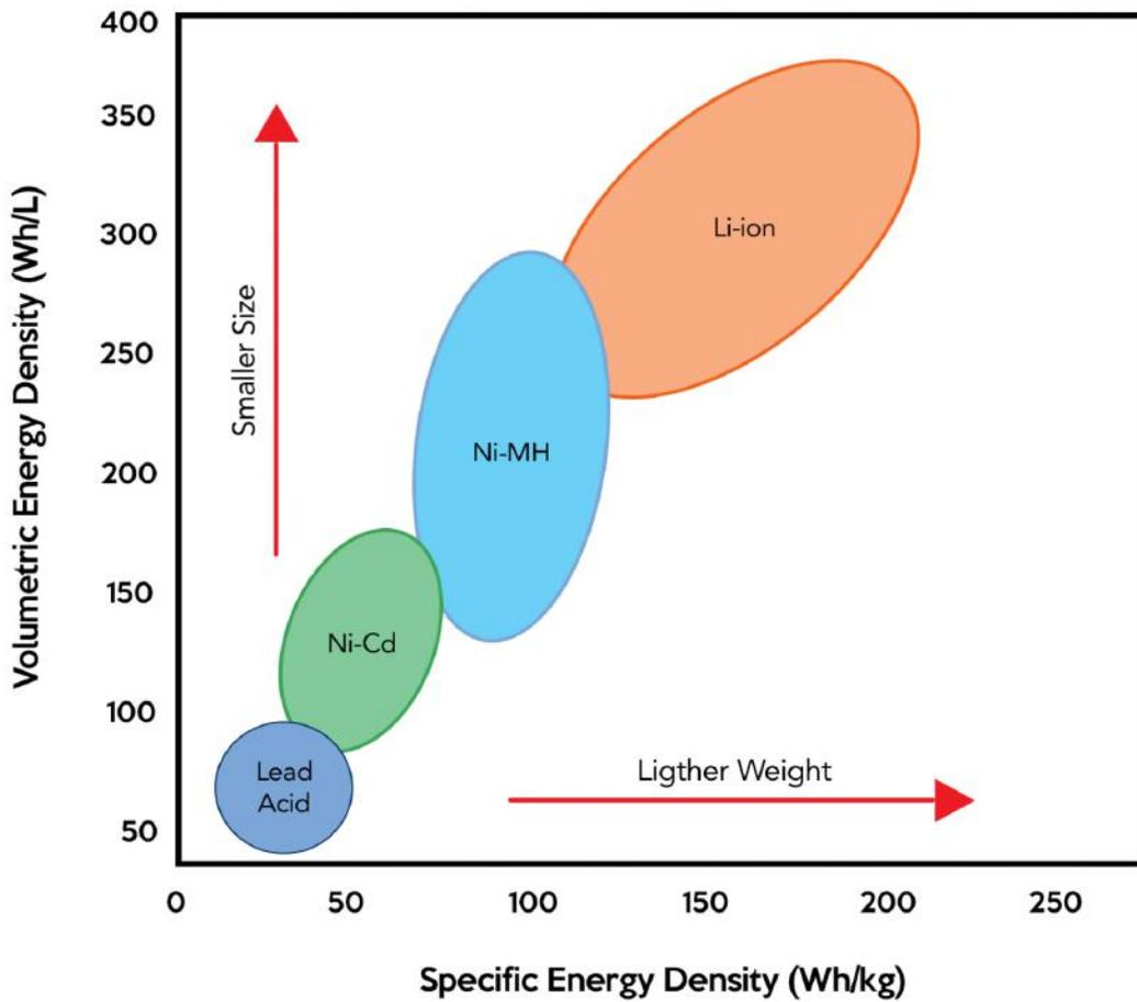
Figure 1: Specific Energy Density, and Volumetric Energy Density of contemporary battery technologies. Source: [NanoPower Research Laboratories](http://NanoPowerResearchLaboratories.com)
