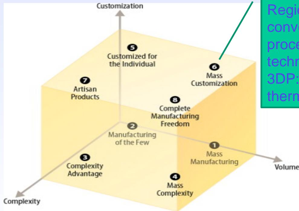
Region 6. Challenging for conventional manufacturing processes. Combined technology processes. 3DP: mold making for thermoplastics
